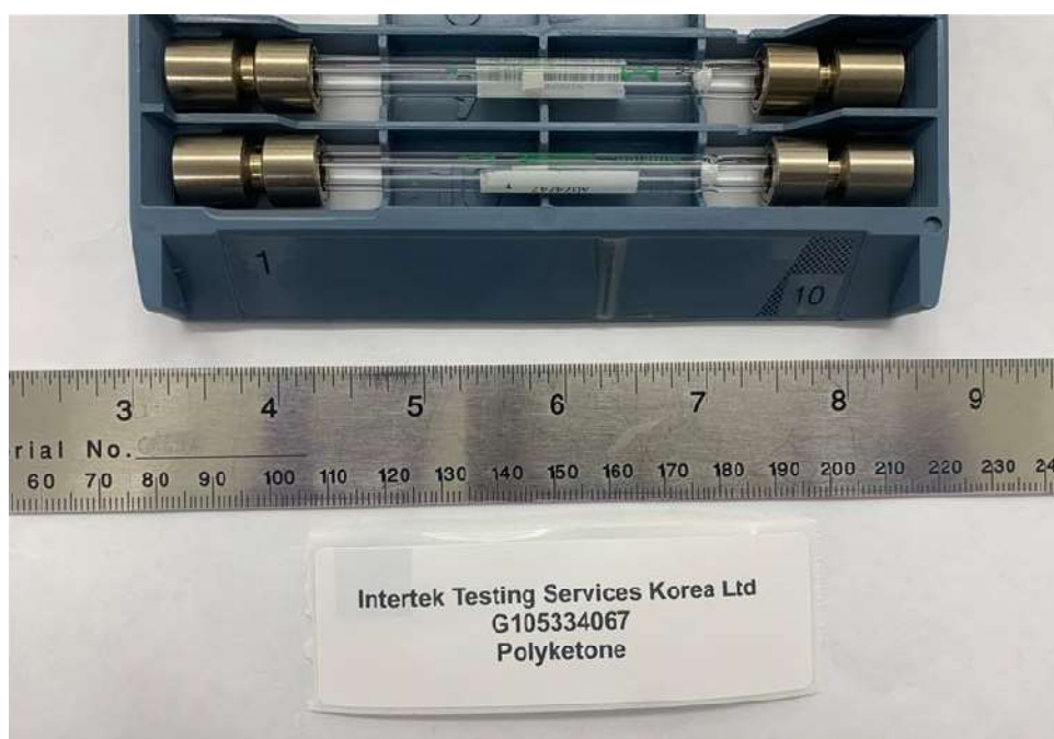
Figure 2: Photograph of Polyketone samples loaded in thermal desorption tubes.
